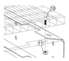
Detail diagram, fastening using J-hook
