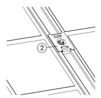
4. Torque tighten the clamp (2) 10 Nm.
