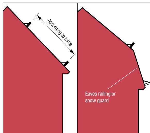
The tables are based on fixings c/c 1200 mm. Distance table for snow guards according to SS 83 13 35:2012 with snow zones according to BFS 2015-6-EKS 10 and form factor according to Eurocode SS-EN 1991-1-3. Loads on load-bearing elements – Parts 1-3: General loads – Snow load.
