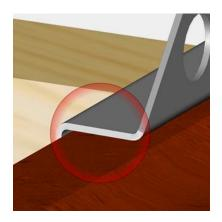
Place the mount on the lath and adjust the height to the underlying roof tile, suitable gap 2-3m, screw the bracket firmly into place with 2 M10x20
