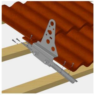
Screw the mount into place using 5 stainless steel wood screws 6x35 as shown in the picture. Fasten the battens, which hold the lath mount, to the trusses using hot dipped galvanised wood screws 125x6.
